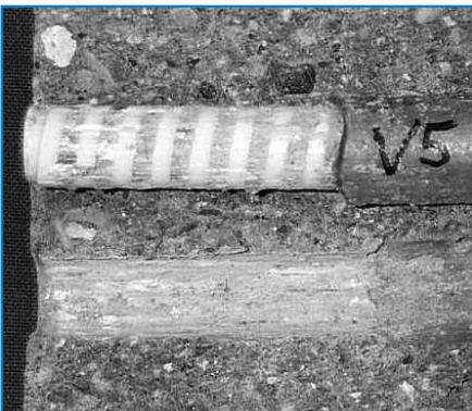
The special surface profile of Schöck ComBAR® bars ensures optimal bond between concrete and the rebar.
