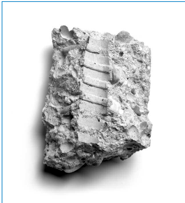
fragment of test specimen showing intact and sheared-off ribs
